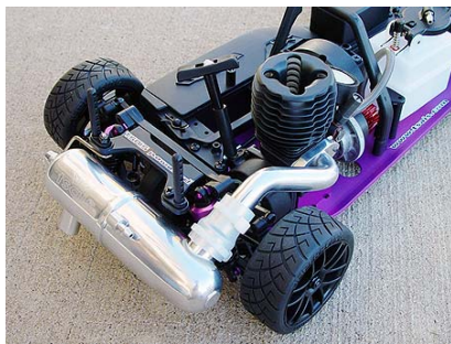
Cut the silicone tube to approximately 32mm (1 1/4") long and then connect the manifold and pipe.
