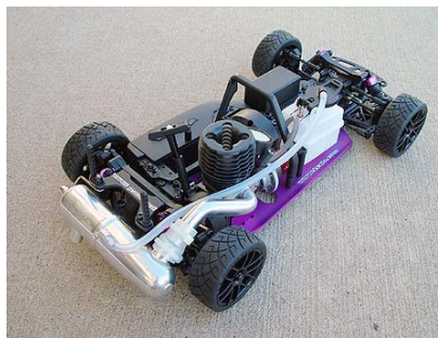
After securing the pipe with zip ties and M4 setscrew. Install the pressure fitting fuel line.
