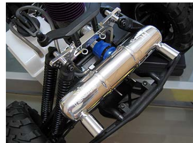
TSAV02 dual rear exhaust pipe and the optional E813 manifold kit shown in picture above.
